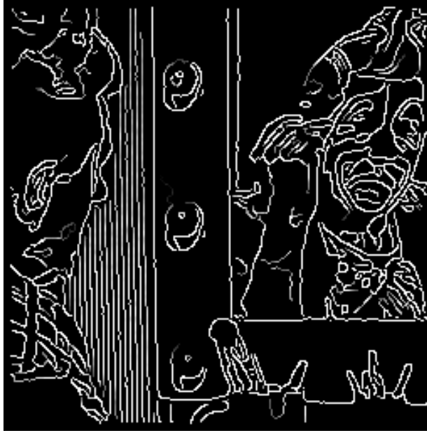
Canny with \sigma = 1
