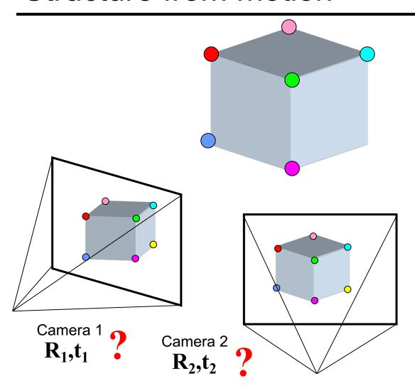
Bootstrapping the process: Given a set of 2D point correspondences in two images, compute the camera parameters
