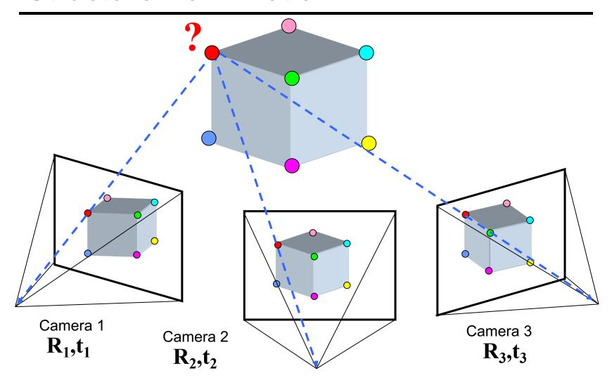
• **Structure:** Given *known cameras* and projections of the same 3D point in two or more images, compute the 3D coordinates of that point
