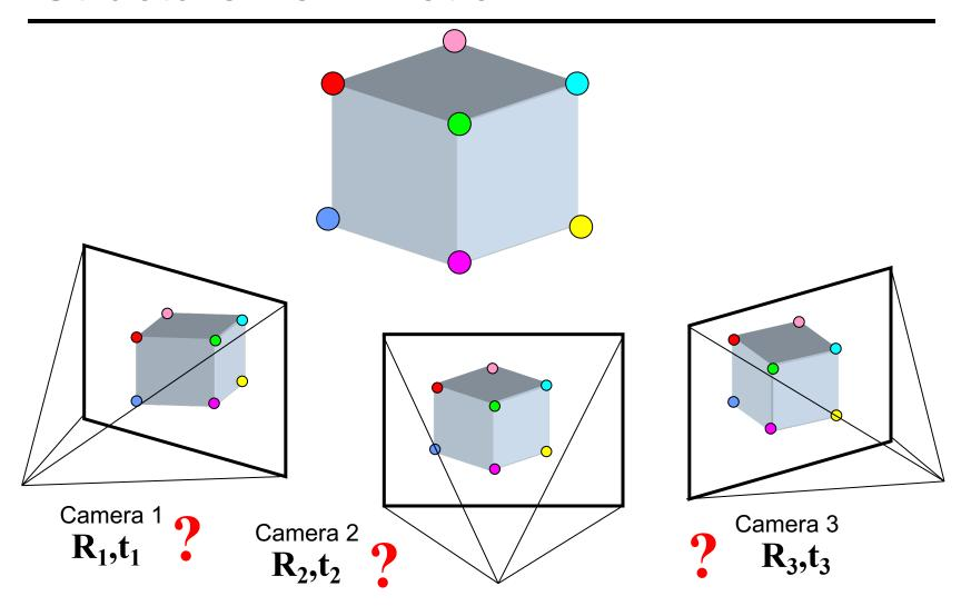
Motion: Given a set of known 3D points seen by a camera, compute the camera parameters
