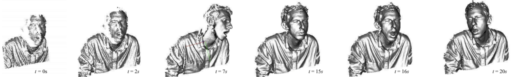
Figure 1: Real-time reconstructions of a moving scene with DynamicFusion; both the person and the camera are moving. The initially noisy and incomplete model is progressively denoised and completed over time (left to right).
